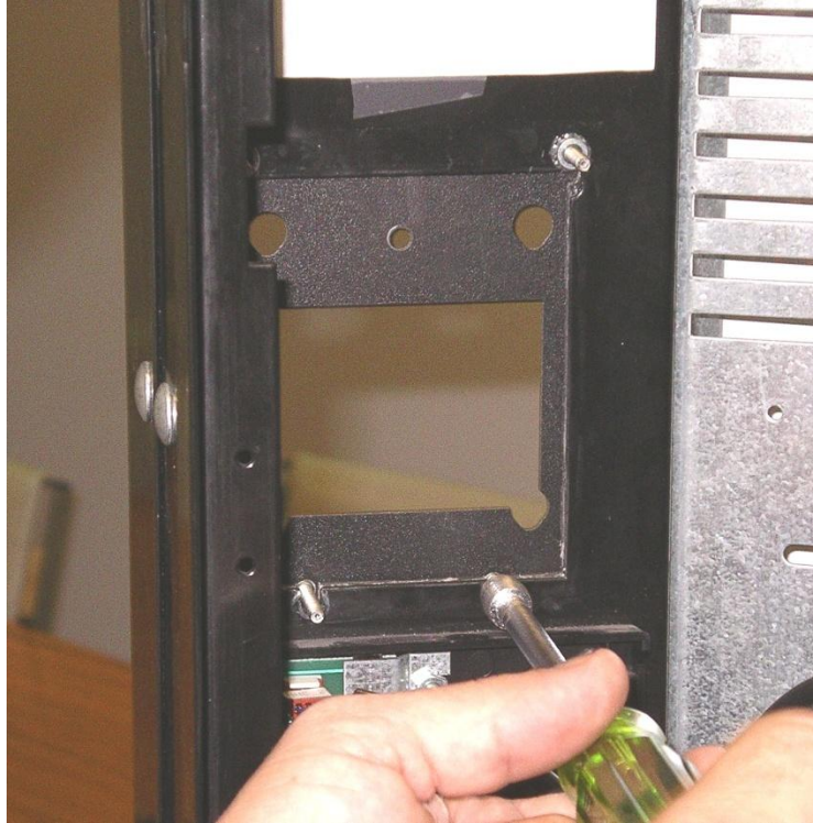
Installing the trim ring nuts (standard shown)
